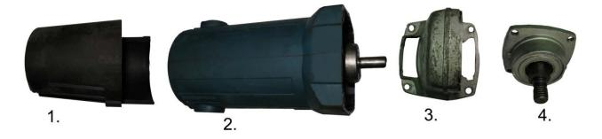
1, rear plastic housing; 2, main body plastic housing; 3, front housing; 4, bearing housing.
